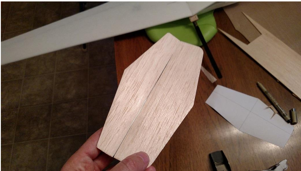
Figure 68: Tape hinge on vertical stab
