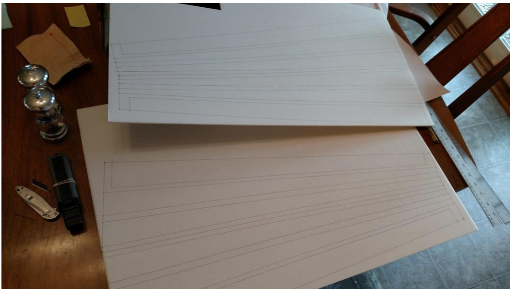
Figure 5: Sheets of DTFB marked up for wings
