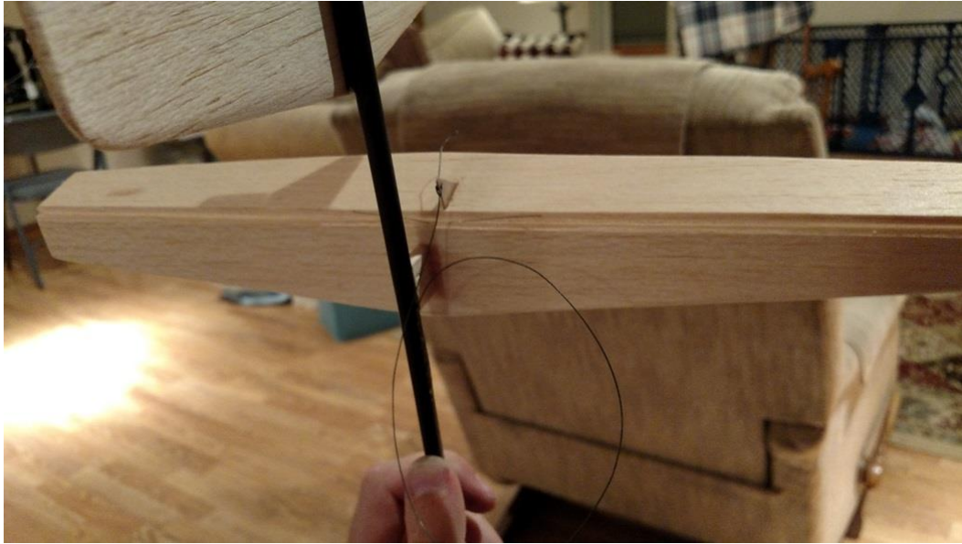
Figure 83: Elevator control string installation through a hole drilled into the tailboom
