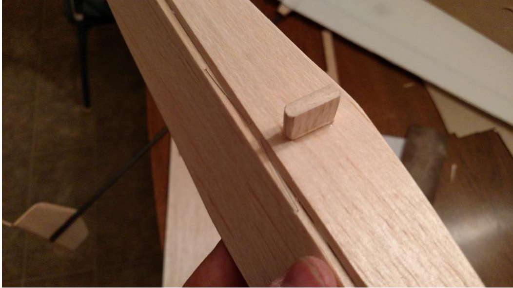
Figure 79: Tail pylon cemented to horizontal stab
