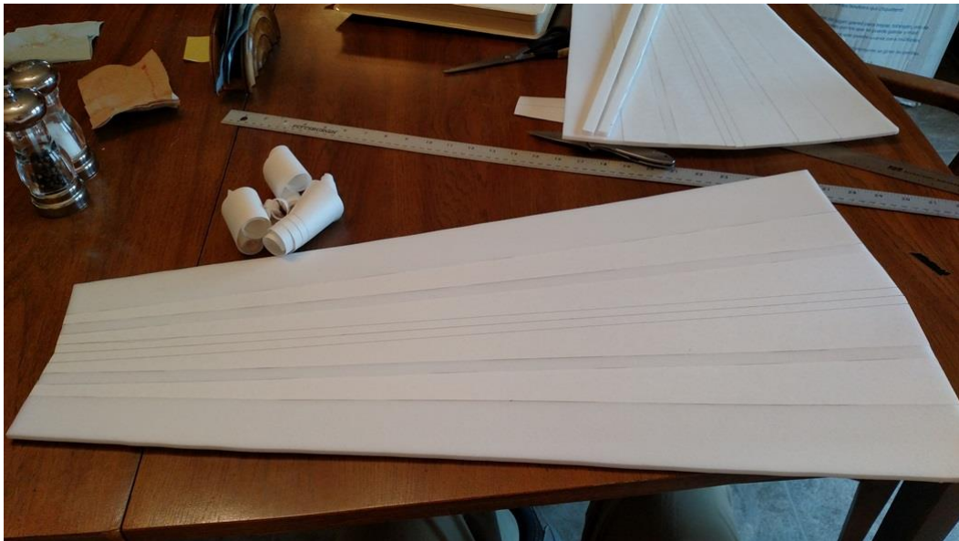
Figure 7: Paper peeled up from flapperons and spar location
