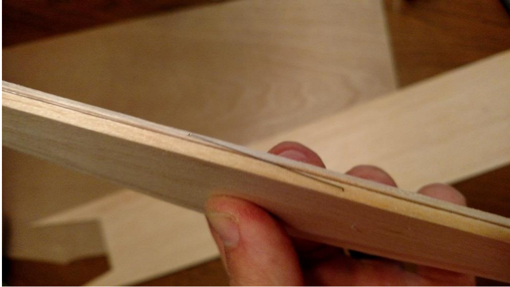
Figure 71: Hinge spring fully installed into vertical stab/rudder
