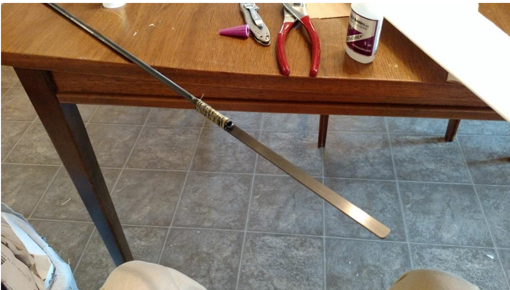
Figure 48: Electronics boom fastened to fuselage boom
