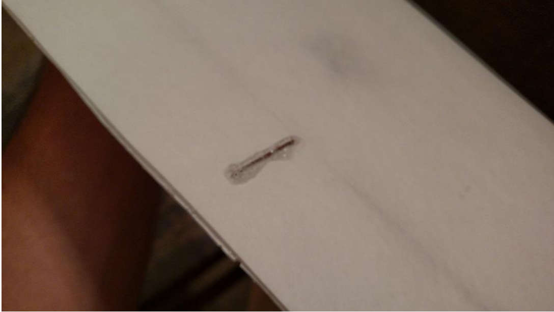
Figure 61: Aileron control horn protruding through top surface and sealed in place
