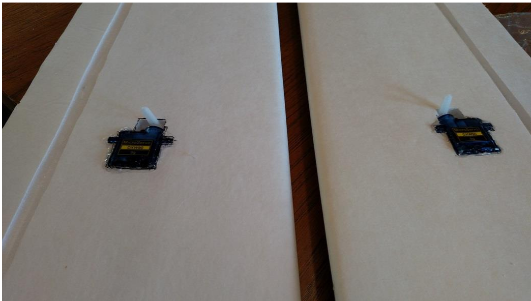
Figure 36: glue fillets around the edges of the servos
