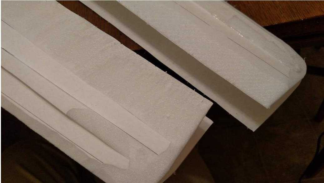
Figure 18: Wing spars tapered at the wingtips
