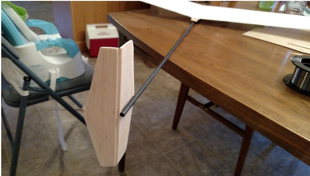
Figure 72: Vertical tail installed for right-handed throwing
