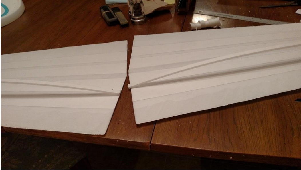
Figure 16: Wing spars peeled on one side each
