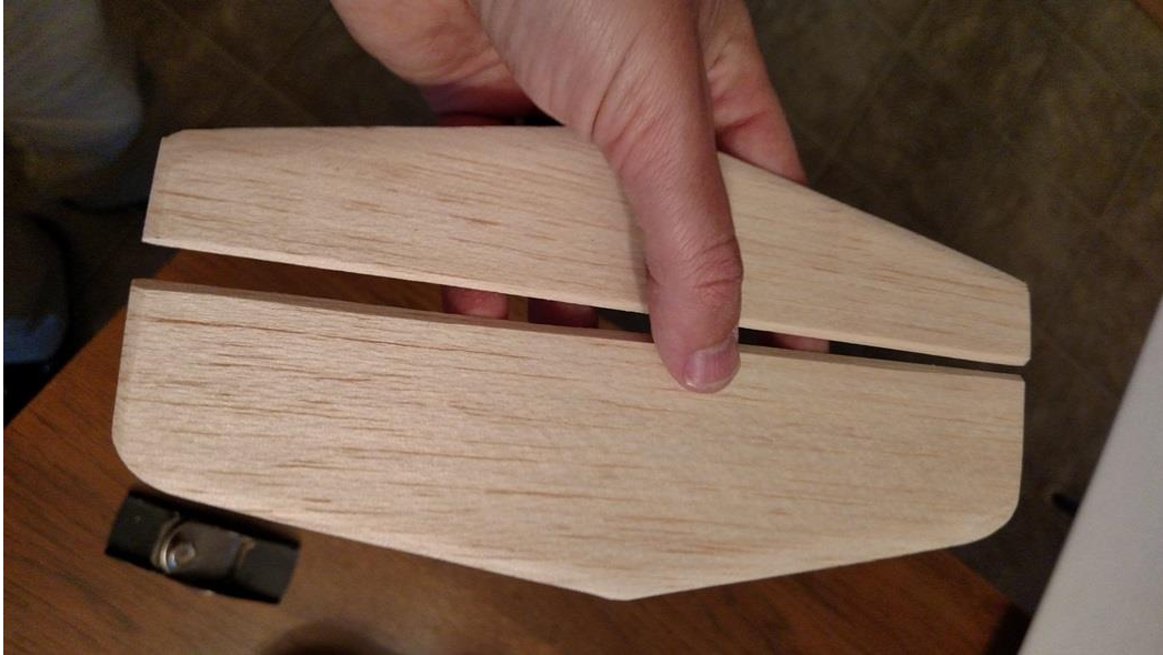
Figure 67: Rudder cut free from vertical stab and beveled for hinge
