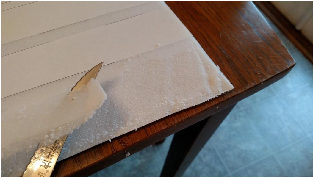
Figure 9: Completing the wing taper
