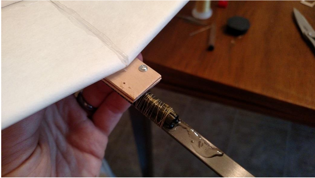
Figure 51: Drilling and screwing the wing in place
