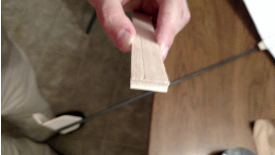
Figure 77: Concave surface sanded into pylon
