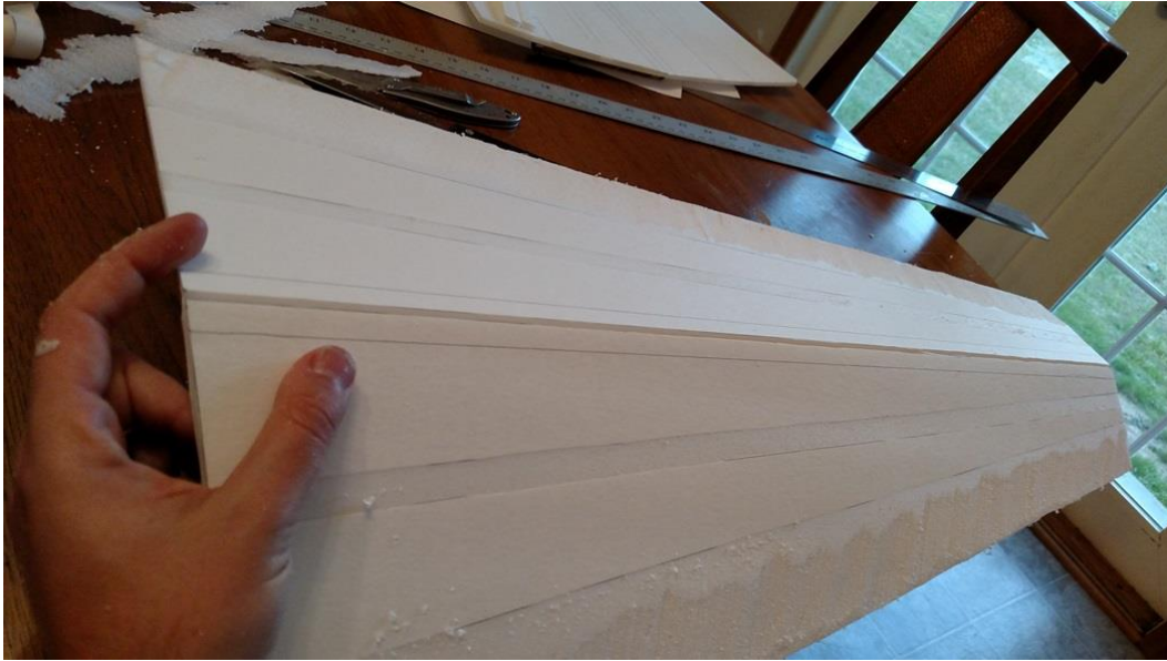
Figure 10: Wing leading edge cut
