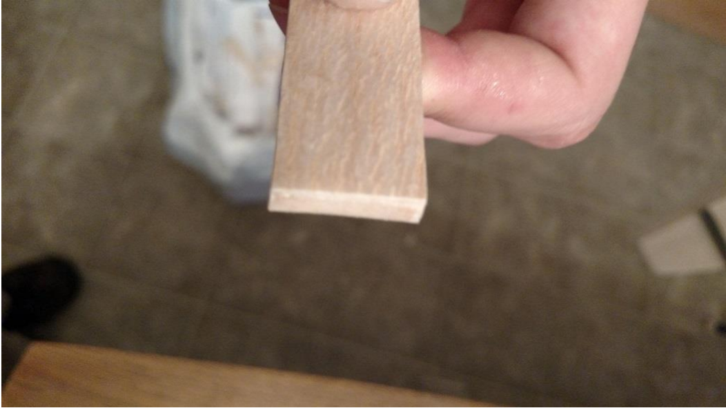
Figure 75: Tail pylon blank cut to width
