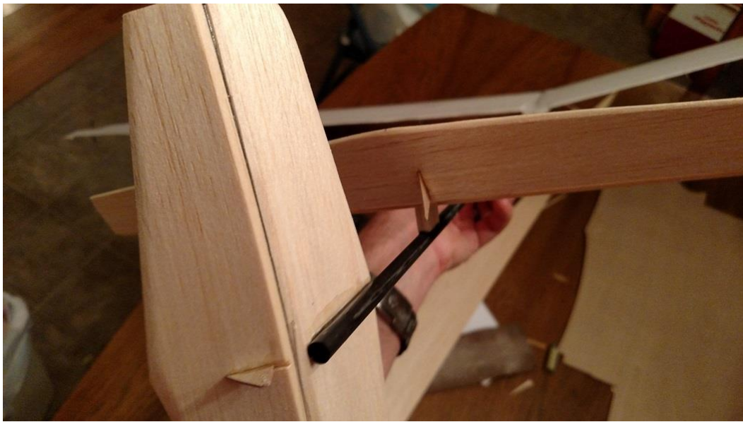
Figure 82: Tail control horns installed
