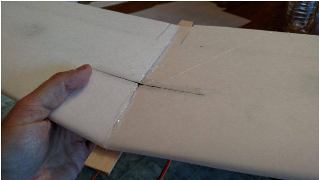
Figure 44: Wing Saddle glued to bottom of the wing, bottom view
