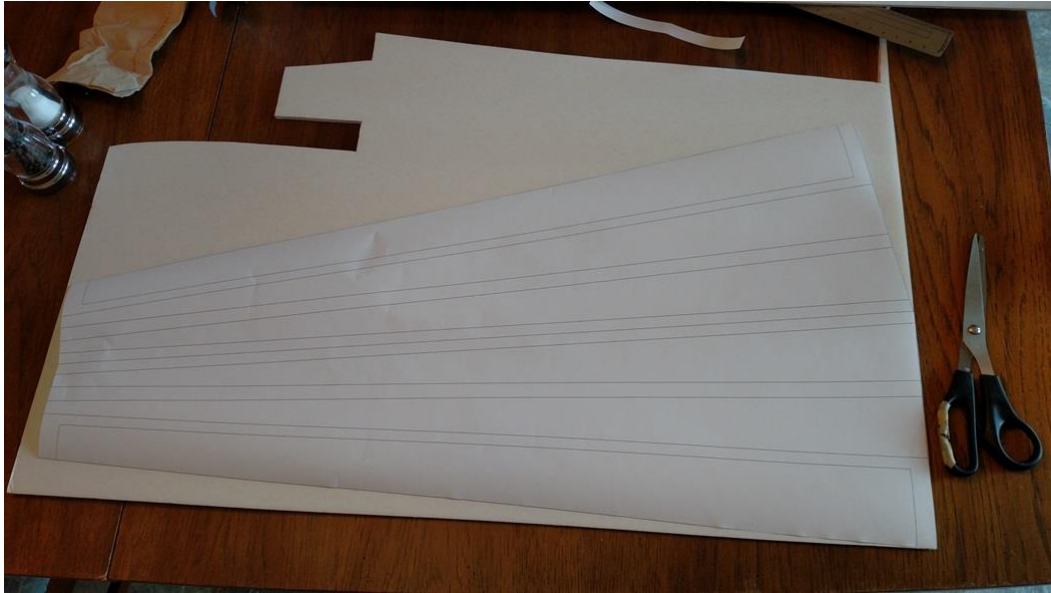
Figure 4: Marking up DTFB for wing construction
