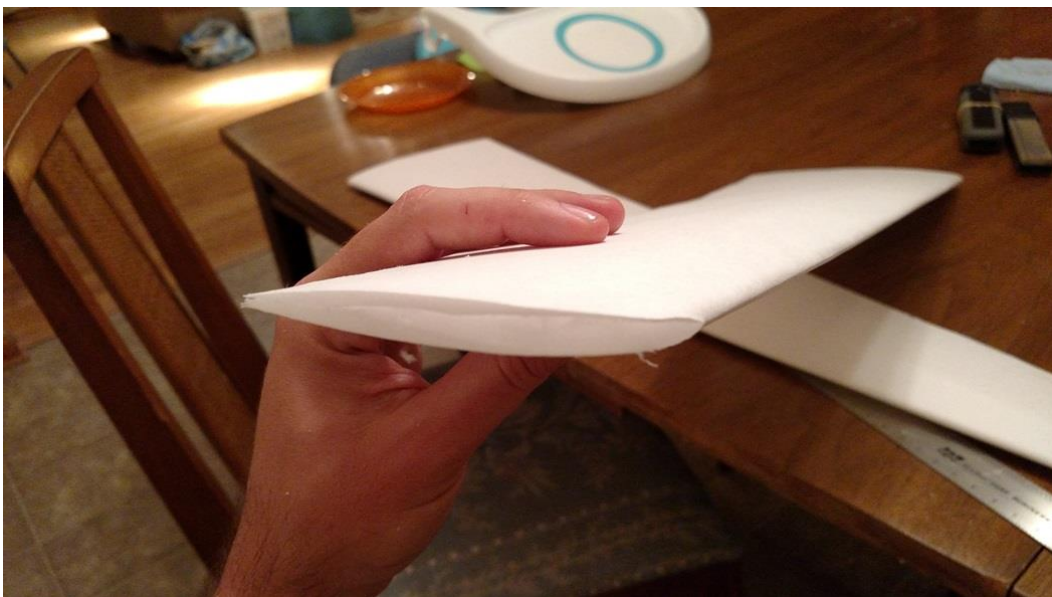
Figure 23: Wingtip still needs to be glued closed
