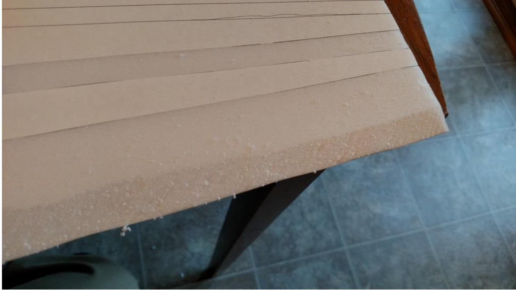
Figure 8: Initial taper of wing trailing edge.
