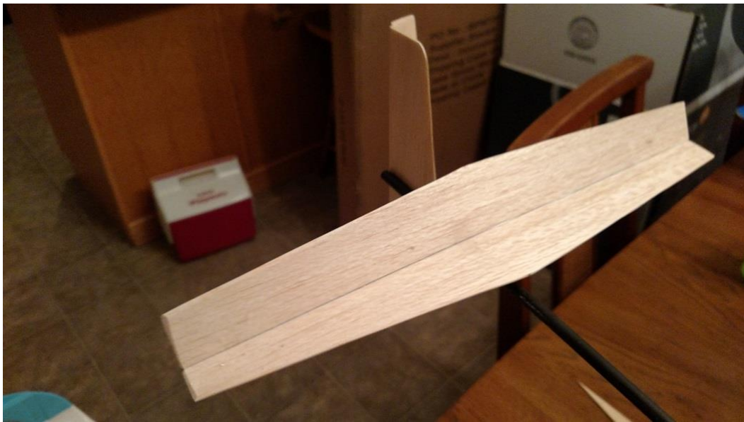
Figure 80: Horizontal stab mounted to top of tailboom
