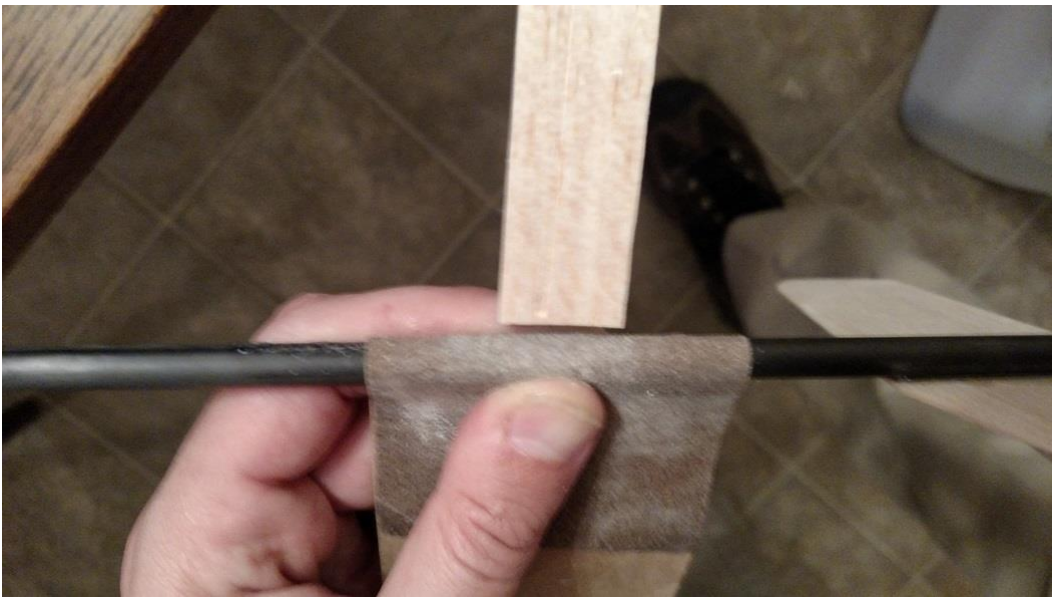
Figure 76: Sanding the pylon's boom mount surface
