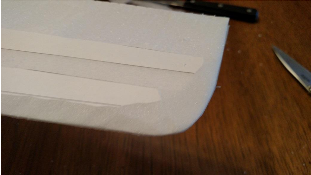
Figure 14: internal taper of wingtip
