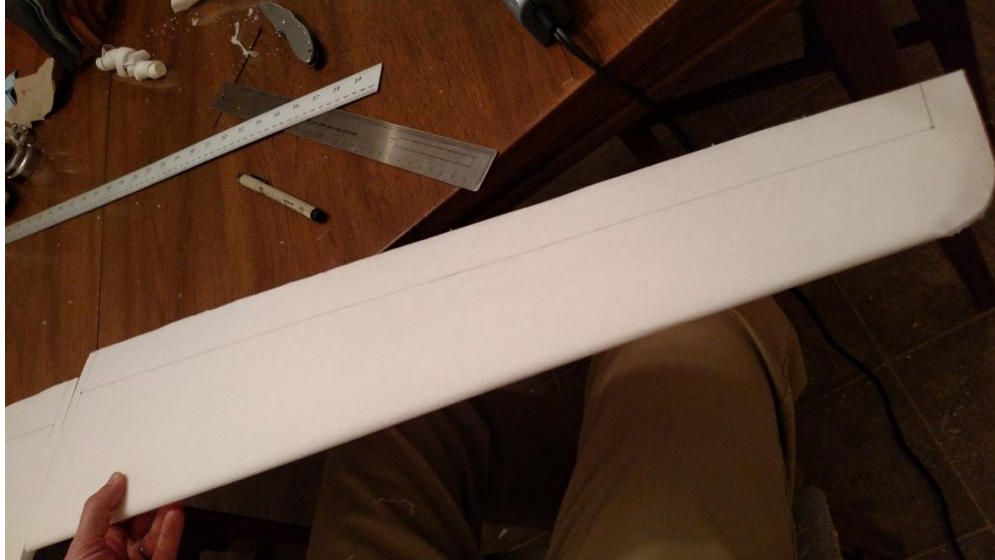
Figure 26: Ailerons marked out on the wings
