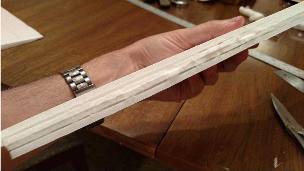
Figure 28: Aileron folded over showing gaps due to incomplete gluing
