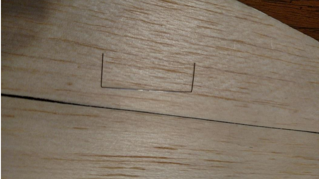
Figure 69: Rudder hinge spring
