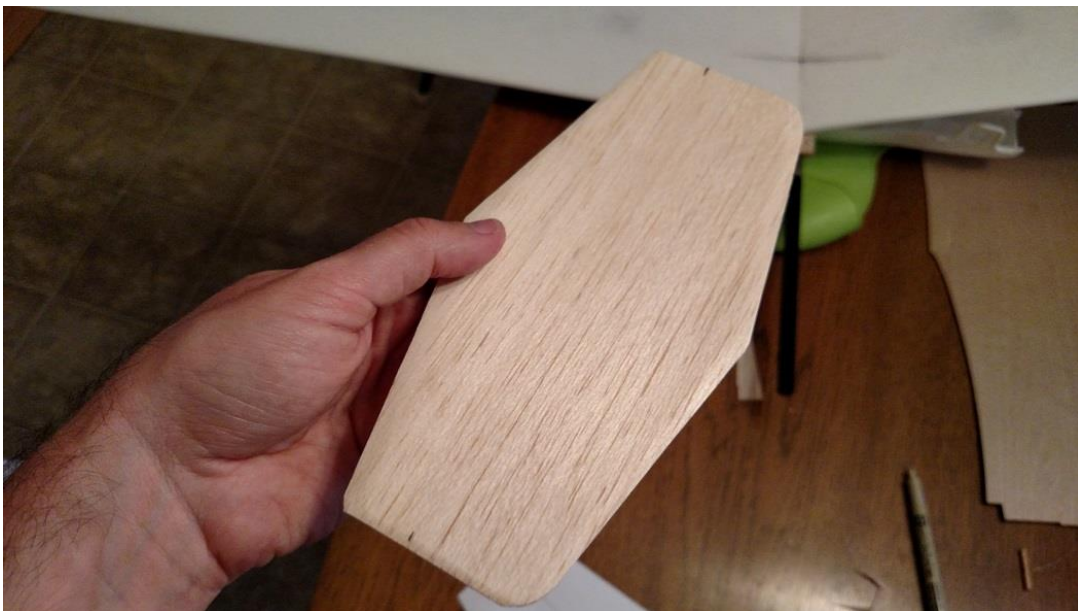
Figure 66: Vertical stab finished and marked for rudder hinge
