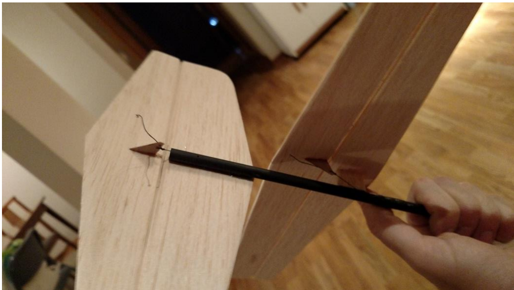
Figure 86: Tail surfaces tensioned into neutral position by servos
