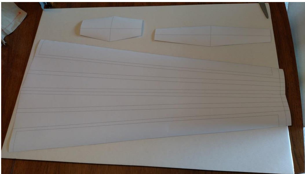
Figure 3: Original plan templates laid out on a sheet of DTFB; note that tail surfaces are not made from DTFB. The wings will not fit together on a single sheet of DTFB unfortunately.
