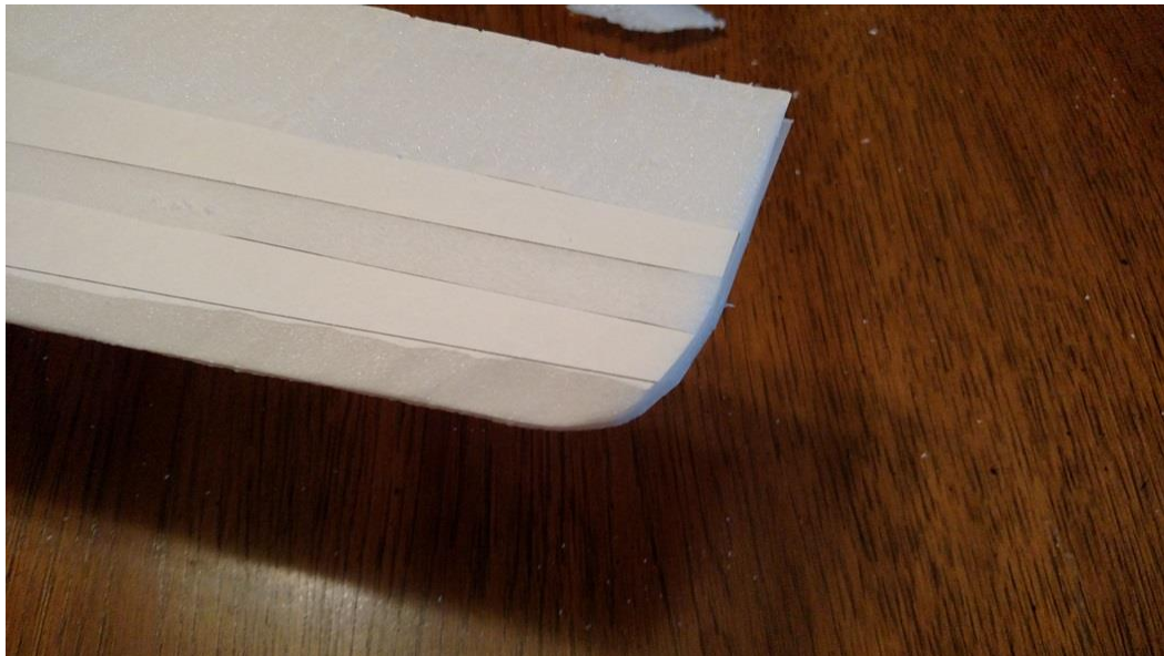
Figure 13: Rounded wingtip leading edges
