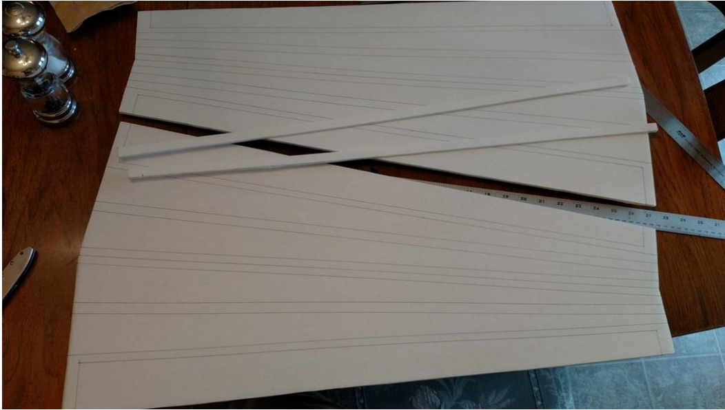
Figure 6: Wing parts cut out from DTFB
