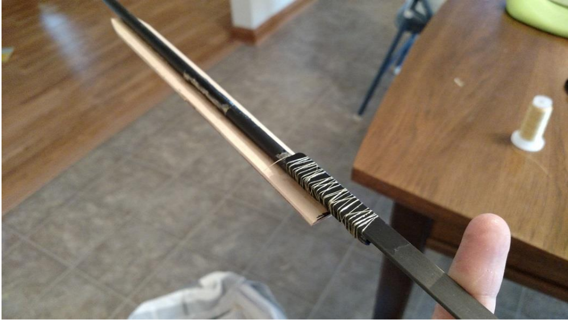
Figure 49: Wing saddle bonded to fuselage, bottom view
