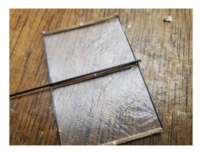
Glue one of the balsa top disks to the top of the vane, sticking the tiny amount of excess carbon rod into the small hole in the disk.
