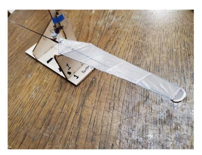
Glue each rib, and the gusset, to the carbon rod. It is not a problem if the gusset has to ride up on the rotor hub in order for the blade to slide fully in place.
