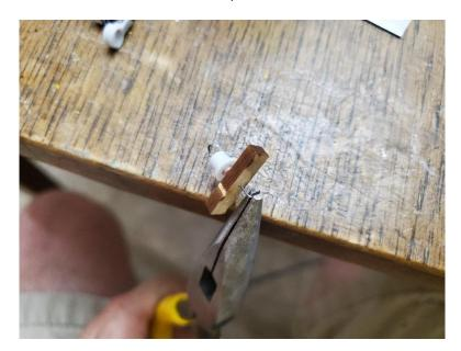
Slide the rotor hub up against the bend and glue the bend over part of the shaft to the hub.
