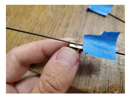
Attach the other 0.040" carbon rod on its centerline at the top of the motorstick where the engraved lines are located below the shrink tube.
