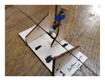
Side a bottom rotor blade in place, covering side up, as shown on the 0.040" carbon rod bottom rotor spar.
