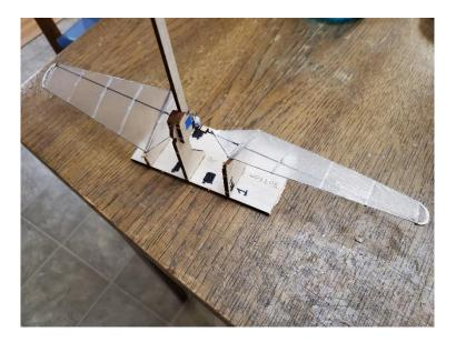
Slide the second bottom rotor blade in place onto the 0.040" carbon rod spar and glue it in place as well.
