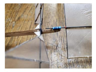
Very carefully slide the second small piece of red tubing onto the bottom of the carbon rod to retain it in the heat shrink tubing.
