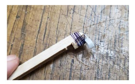
Locate a rotor bearing assembly (prop shaft, bearing, washer) and a **bottom rotor** hub. Note that in the photo below, a small piece of masking tape has been added to the bearing to make it fit in the bearing mount more tightly while still being removable for storage/repair.
