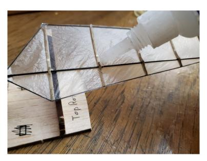
Without removing the assembly from the jig, install the **second top rotor blade** by repeating the above steps and verifying with the photo below.
