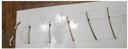
Lay in place one of the 0.020" carbon rods (these are the thin rods). Use scissors or wire cutters to trim the other end of the carbon rod. DO NOT throw away the excess carbon—you will need it later!
