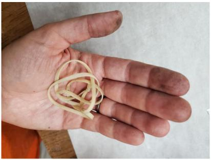
You can now load the rubber onto the rear hook and the prop shaft. Typically the rubber will be very slack, hanging loose under the model. It's ok for the rubber to hang loose, as this will actually reduce tension on the prop bearing and allow the rubber to be wound more tightly.
