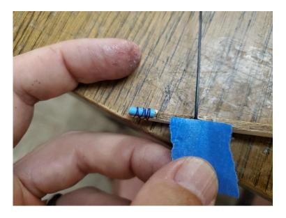
Remove the tape and bind the rod firmly in place with thread and harden with glue.
