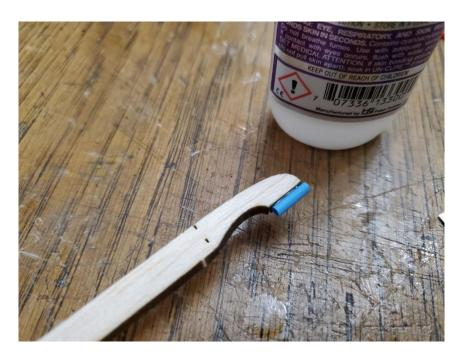
Bind the tubing in place with thread and harden the thread with glue, being careful to avoid getting any glue in side the tube.
