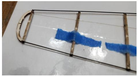
You can now remove the tape strips and carefully remove the blade from the plans.
