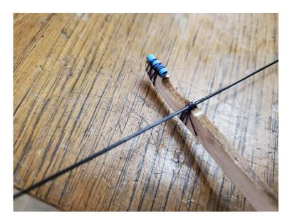
Attach a pair of gussets on either side of the motorstick as shown to reinforce the rod attachment.
