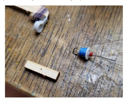
Slide the rotor hub onto the propeller shaft.
