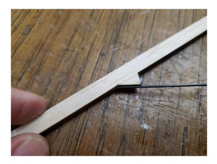
Bind the rod in place and harden with glue. Trim off the excess thread.
