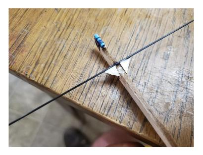
Insert the top end of the motorstick into the top rotor jig as shown, using the side plate in the motorstick mast to hold the motorstick in place. Tape the motorstick in place for additional retention. DO NOT GLUE THE MOTORSTICK TO THE MAST OR THE REST OF THE JIG!!!
