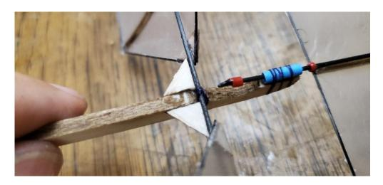
**Congratulations!!!** Your Tornado 2024 is now complete! Weigh your model to verify that it meets the minimum weight of 4.00g. If not, glue clay to the bottom of the motorstick, out of the way of the propeller shaft and rotor, to bring it up to the minimum weight.
