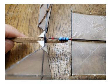
Use a **tiny drop** of glue on the **bottom** of the red tubing to secure it to the carbon rod.
