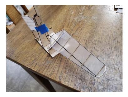
Remove the completed motorstick/top rotor assembly from the top rotor jig.
