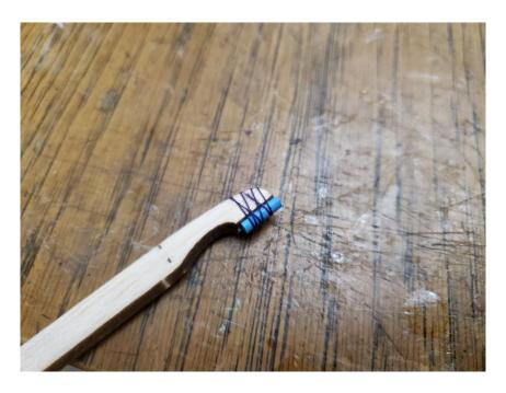
Find a piece of 0.040" carbon rod, and line it up with the triangular protrusion (called a gusset) on the motorstick.
