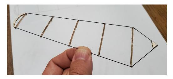
Repeat the above steps to finish a second bottom rotor blade. The use the top rotor template to build two top rotor blades.
