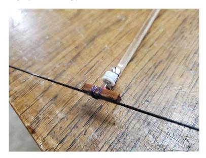
Slide the bottom rotor/motorstick assembly into the bottom rotor jig as shown, sliding the motorstick downward until the 0.040" carbon rod spar contacts the jig at the laser cut slots. Use a piece of tape to secure the motorstick in place on the bottom motorstick mast. Do not glue the motorstick in place!
