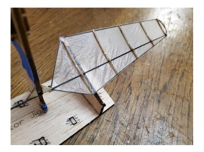
Glue each rib to the carbon rod with a small drop of glue. Don't forget to glue the gusset to the carbon rod as well.
