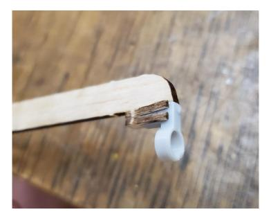
Bind the bearing firmly in place on the bottom end of the motorstick with thread, harden the thread with glue, and trim off the excess.
