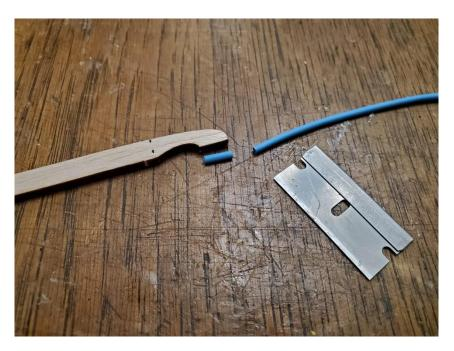
Glue the tubing in place on the flat of the motorstick (top end).
