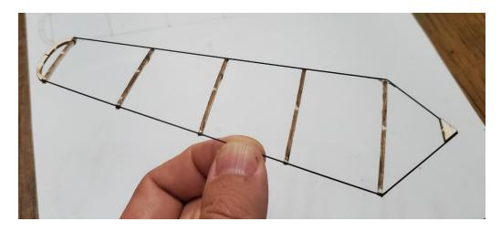
Repeat the above steps to finish a second bottom rotor blade. The use the top rotor template to build two top rotor blades.
