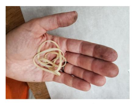
You can now load the rubber onto the rear hook and the prop shaft. Typically the rubber will be very slack, hanging loose under the model. It's ok for the rubber to hang loose, as this will actually reduce tension on the prop bearing and allow the rubber to be wound more tightly.
