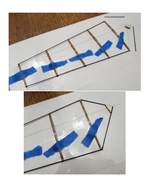
You can now remove the tape strips and carefully remove the blade from the plans.
