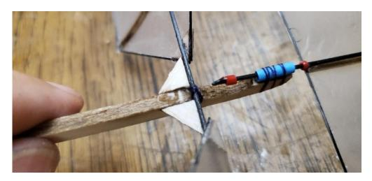
**Congratulations!!!** Your Tornado 2024 is now complete! Weigh your model to verify that it meets the minimum weight of 4.00g. If not, glue clay to the bottom of the motorstick, out of the way of the propeller shaft and rotor, to bring it up to the minimum weight.
