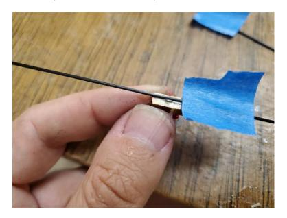
Wrap the hub/carbon rod joint with thread and harden with glue.
