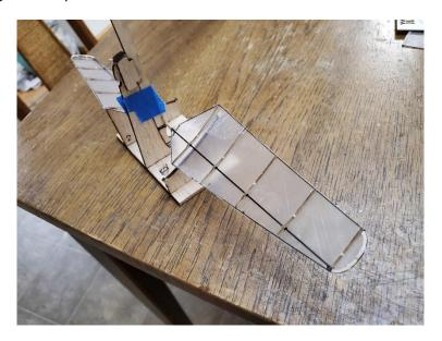
Remove the completed motorstick/top rotor assembly from the top rotor jig.
