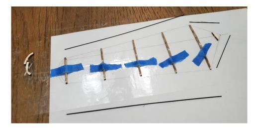
The ribs have small notches on the ends to fit the carbon outline. Glue the ribs to the carbon outline. Take your time to try to get them aligned as closely as possible over the rib marks on the template.
