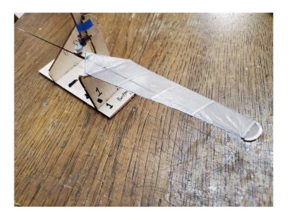
Glue each rib, and the gusset, to the carbon rod. It is not a problem if the gusset has to ride up on the rotor hub in order for the blade to slide fully in place.
