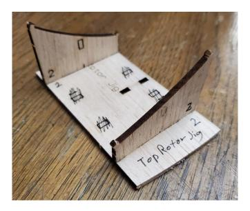
Remove the **top rotor** motorstick post from the jig sheet and attach the side plates to it as shown.
