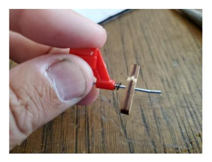
Bend the end of the shaft over at a SHARP 90 degree angle as shown. If your fingers do not hurt when you are bending the wire over, you're not pressing hard enough, and you will end up with a curved propeller shaft which doesn't turn true. Bend it sharp and neat!
