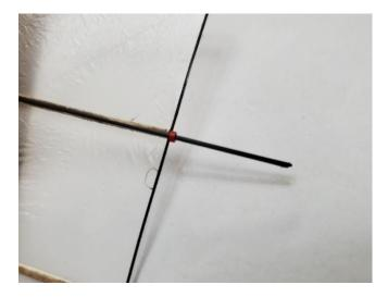
Slide the end of the carbon rod into the heat shrink tubing on the top of the motorstick.
