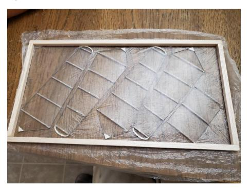
Use an electric cautery (available from indoorffsupply.com) or brand new razor blade to cut the film around the outside of the flying surfaces. Do not leave any excess. Try to get as smooth of a trimming job as possible. Excess film waving in the air will make your model fly poorly.
