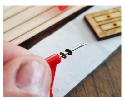
Slide a wooden rotor hub onto the propeller shaft.
