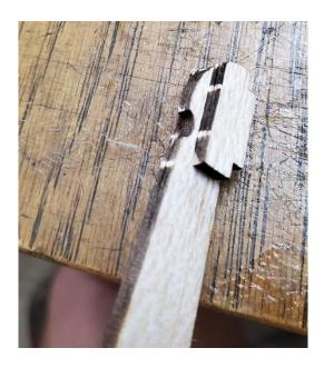
Attach the **top rotor** motorstick post to the jig exactly as shown below. **This orientation is absolutely crucial!**
