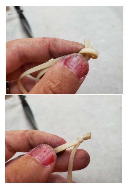
Tie a second granny knot and sinch it up to the first one for added security. Add a tiny dab of glue to the knot on the outside (free ends) of the rubber loop. Trim off any excess.
