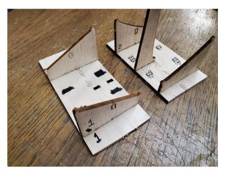
Assemble the **bottom rotor** motorstick post with its side plates as shown.
