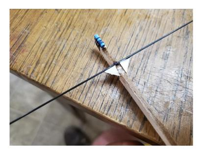
Insert the top end of the motorstick into the top rotor jig as shown, using the side plate in the motorstick mast to hold the motorstick in place. Tape the motorstick in place for additional retention. DO NOT GLUE THE MOTORSTICK TO THE MAST OR THE REST OF THE JIG!!!
