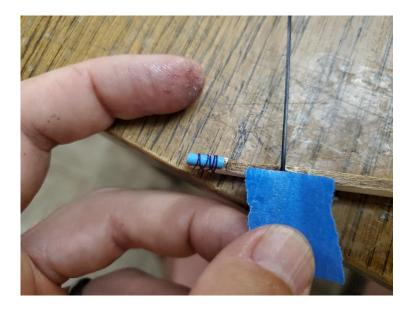
Remove the tape and bind the rod firmly in place with thread and harden with glue.
