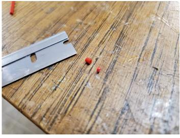
Slide one of the red plastic tubing pieces onto the rotor vane mast as shown. It does not need to be glued in place.
