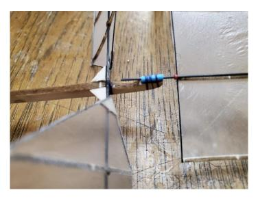
Very carefully slide the second small piece of red tubing onto the bottom of the carbon rod to retain it in the heat shrink tubing.
