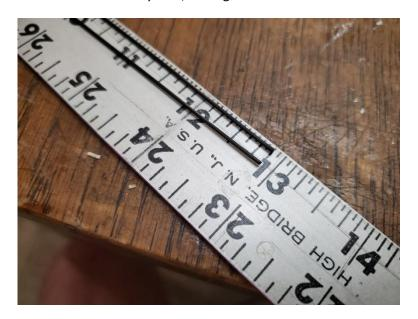
Place a piece of masking tape on each rod at the 6 7/16" point as shown to mark their center lines.
