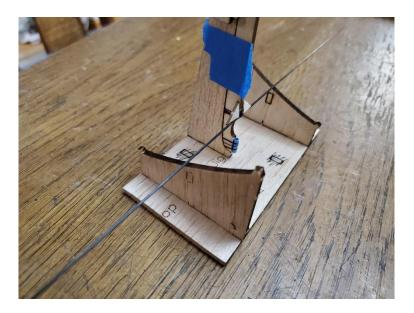
Slide a **top rotor blade** onto the 0.040" carbon rod as shown (covered side down) until the rod is flush with the outside edge of the outermost rib. You may need to sand the ends of the carbon rod to get it to slide into the ribs reliably. Take your time on this step as it is easy to break the ribs in the process!
