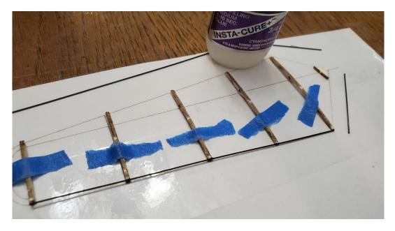
Continue attaching the carbon outlines as shown. Note that the triangular gusset at the root end of the blade is used to reinforce that joint. The optional blade tip should be assembled and added at this time.
