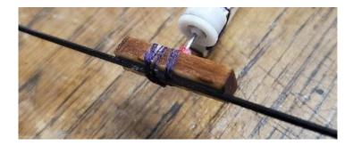
Attach the other 0.040" carbon rod on its centerline at the top of the motorstick where the engraved lines are located below the shrink tube.
