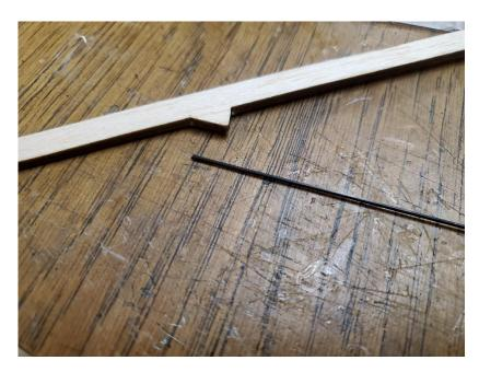
Line the 040" carbon rod with the gusset and press it into the motorstick parallel to the face of the gusset. The rod should point upward to toward the shrink tubing end of the motorstick. Glue it firmly in place.
