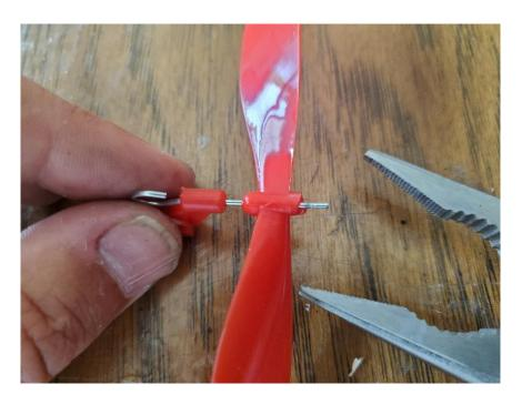
Remove the propeller and set it aside. It cannot be used for Science Olympiad competition per the rules requiring student-built rotors.
