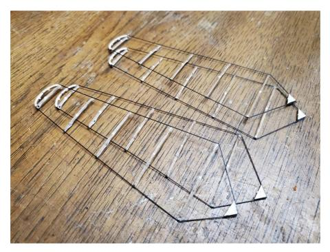
Use the same procedures to build the **Rotor Vane** using the rotor vane ribs, 0.020" carbon rods, and rotor vane template.
