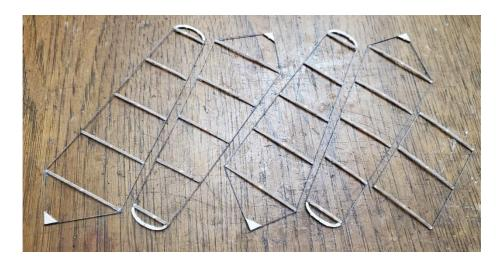
Lay the parts, adhesive side up, onto a smooth, flat surface. Carefully lower the covering frame, covering side down, onto the flying surfaces. Then gently run your finger around the outlines of the wing and tail to press the film into contact with the parts. Be careful to press very, very gently so that you do not damage the fragile ribs!
