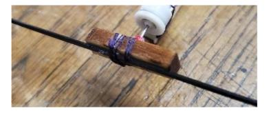
Attach the other 0.040" carbon rod on its centerline at the top of the motorstick where the engraved lines are located below the shrink tube.
