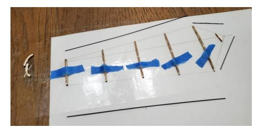
Glue the ribs to the carbon outline. Take your time to try to get them aligned as closely as possible over the rib marks on the template.
