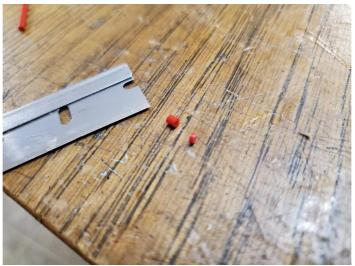
Slide one of the red plastic tubing pieces onto the rotor vane mast as shown. It does not need to be glued in place.
