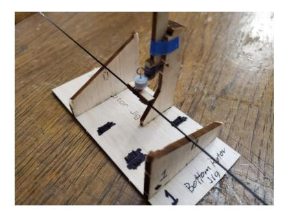
Side a bottom rotor blade in place, covering side up, as shown on the 0.040" carbon rod bottom rotor spar, up to the second rib as you did on the top rotor.
