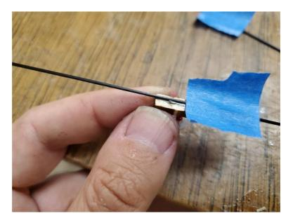
Wrap the hub/carbon rod joint with thread and harden with glue (Ikara grey bearing shown in photo).
