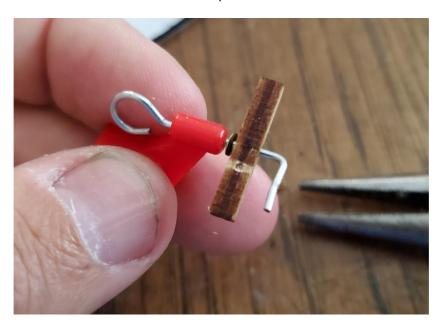
Slide the rotor hub up against the bend and glue the bend over part of the shaft to the hub.
