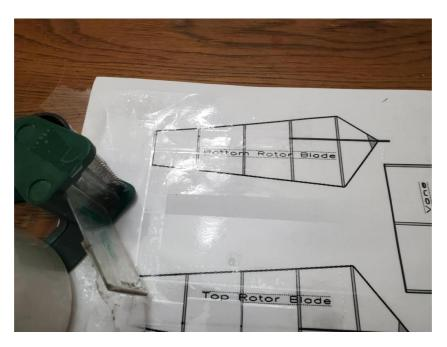
Warning: the patterns are labeled Top and Bottom for the rotor blades. You will need to build two (2) top blades and two (2) bottom blades. If you fail to follow this process, your helicopter WILL NOT FLY. Such mistakes will require you to purchase additional parts to produce a flyable helicopter.
