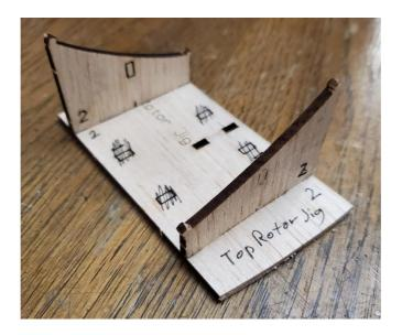
Remove the **top rotor** motorstick post from the jig sheet and attach the side plates to it as shown.
