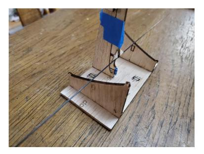
Slide a **top rotor blade** onto the 0.040" carbon rod as shown (covered side down) until the rod is flush with the outside edge of the second rib (only two ribs have holes for the spar). You may need to sand the ends of the carbon rod to get it to slide into the ribs reliably. Take your time on this step as it is easy to break the ribs in the process!
