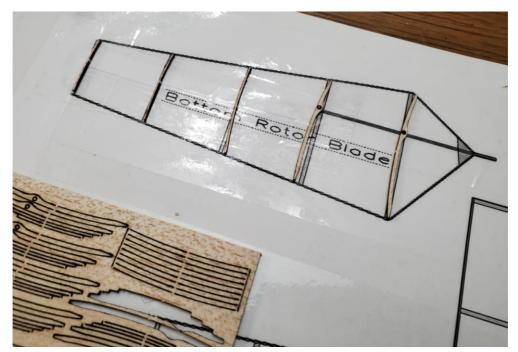
Lay in place one of the 0.020" carbon rods (these are the thin rods). Use scissors or wire cutters to trim the other end of the carbon rod. DO NOT throw away the excess carbon—you will need it later!
