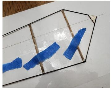
You can now remove the tape strips and carefully remove the blade from the plans.
