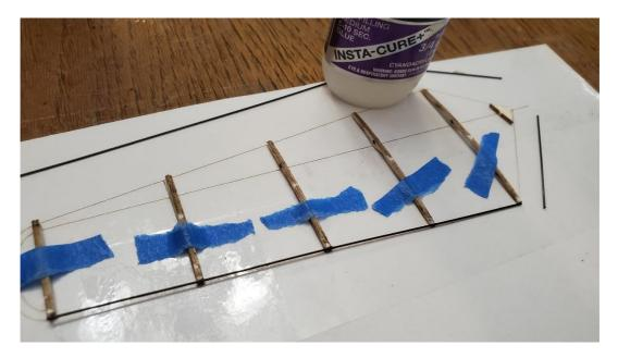
Continue attaching the carbon outlines as shown. Note that the triangular gusset at the root end of the blade is used to reinforce that joint.
