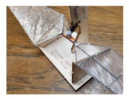
Slide the second bottom rotor blade in place onto the 0.040" carbon rod spar and glue it in place as well.
