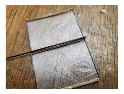
Glue one of the balsa top disks to the top of the vane, sticking the tiny amount of excess carbon rod into the small hole in the disk.
