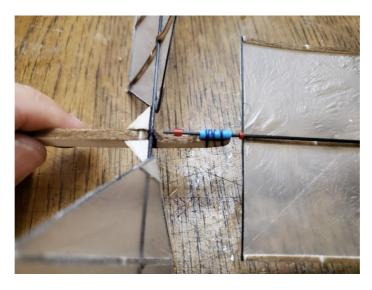
Use a **tiny drop** of glue on the **bottom** of the red tubing to secure it to the carbon rod.
