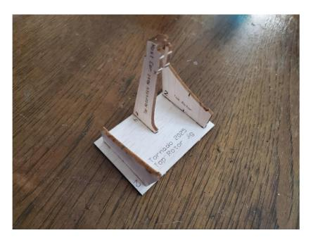
Assemble the bottom rotor jig as shown, matching up the numbers to achieve the mirror image of the top rotor jig as shown.
