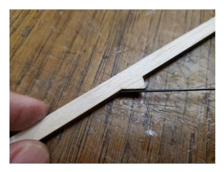
Bind the rod in place and harden with glue. Trim off the excess thread.
