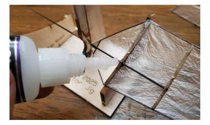
Without removing the assembly from the jig, install the **second top rotor blade** by repeating the above steps and verifying with the photo below.
