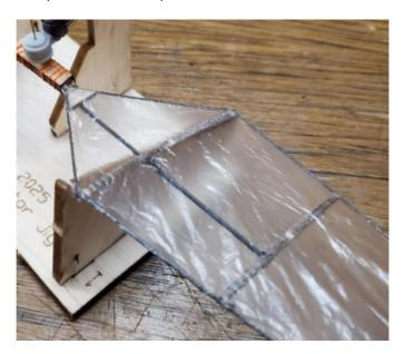
Glue each rib, and the gusset, to the carbon rod. It is not a problem if the gusset has to ride up on the rotor hub in order for the blade to slide fully in place.
