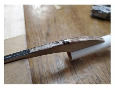
You should now check the fit of your nose cone to the motor tube. If it has a tight fit, carefully sand the nose cone shoulder until it slides in and out easily, but does not fall out on its own if the nose of the model is pointed straight down. Harden the back of the nose cone shoulder with epoxy to prevent erosion of that area by the hot ejection gases. Do not glue the nose cone into the motor tube! It must remain free to be ejected from the nose of the rocket at the end of the engine burn.
