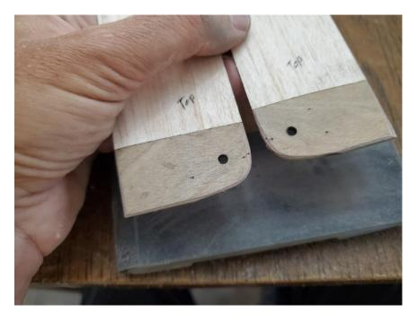
You will now carefully insert the plastic bearings from the bottom of the wings. Test fit to verify that they fit correctly and to understand their alignment before adding glue. After adding glue, you will need to carefully press the bearing in place so that it stays aligned with the hole. Refer to the photo to ensure that you insert the bearing in the correct direction. CA glue and epoxy are the only adhesives recommended for attaching the bearings.
