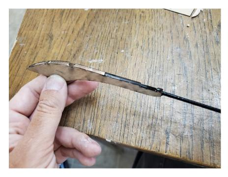
Install the saddle. Once the glue has hardened, bind the joint with the supplied Spider Wire line and fill the binding with CA. If you are uncomfortable with CA, use 5-15 minute epoxy to mount the saddle; binding may be added before the glue has set up; you will need to jig the saddle to ensure that alignment is retained. Before either type of glue has hardened, it is important to ensure that the saddle is correctly aligned.
