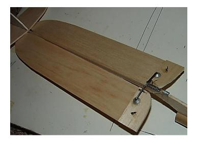
Loop the free end of the Spiderwire through the remaining wing hold down-loop shown and remove all slack from the line.
