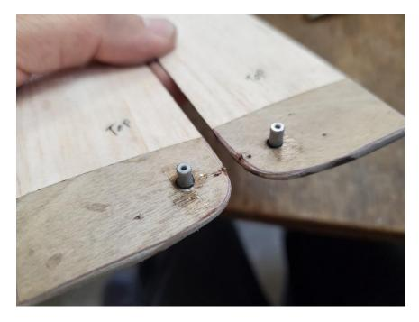
Install the wire hooks and loops as shown. Pay close attention to the angle of attachment of the hooks so that the rubber band will correctly attach and open the wings.
