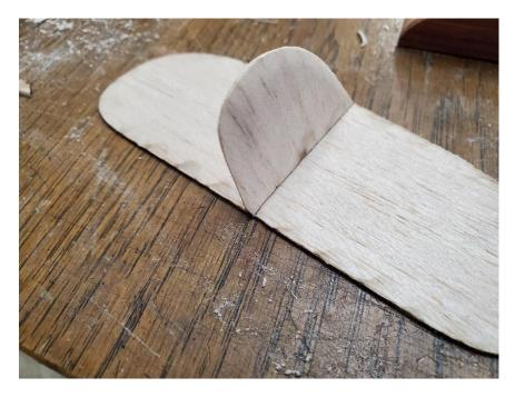
Glue the wedge against the fin with the thick end toward the back.
