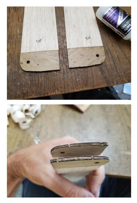
Sand the wing pads to shape and remove any burrs.
