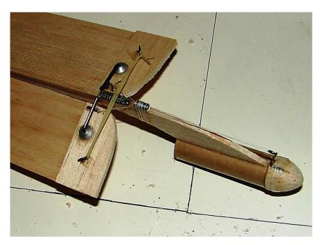
Slide the nose cone out of the front of the motor tube and release it to verify that the wings deploy fully and correctly. Note that the wings are still free to be removed from the hinge saddle. Take a moment to verify that when viewed from the front, your wings are aligned correctly. If they are not aligned together, you will need to twist one of the hinge saddle wires forward or backard to achieve correct alignment. Be careful to avoid bending the hinge axle
