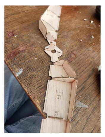
The bottom rotor jig (Sheet #3/#4) is exactly the reverse of the top sheet. Install its parts as a complete mirror image of the top rotor jig.
