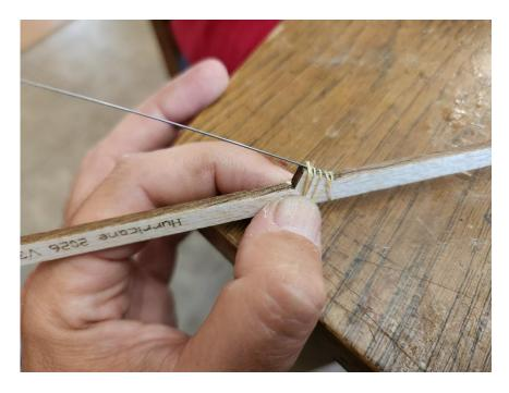
Bend the wire out from the motorstick, back, and cut to size.
