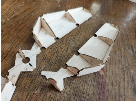
Join the bottom rotor jig halves together in the same manner as the top jig.
