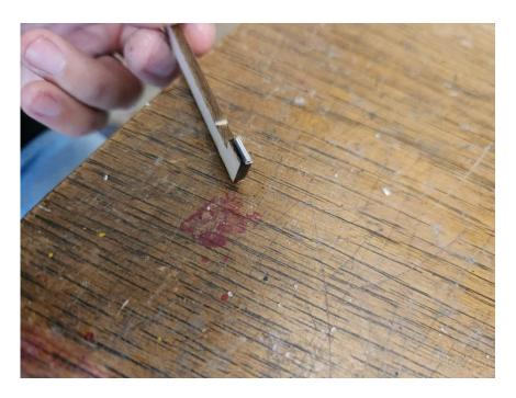
Bind the tubing firmly in place with thread and harden with CA glue, being careful not to get any glue inside the tube.
