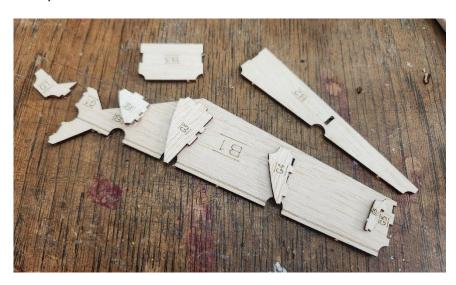
Assemble the jig as shown, making sure all of the tabs are fully inserted.
