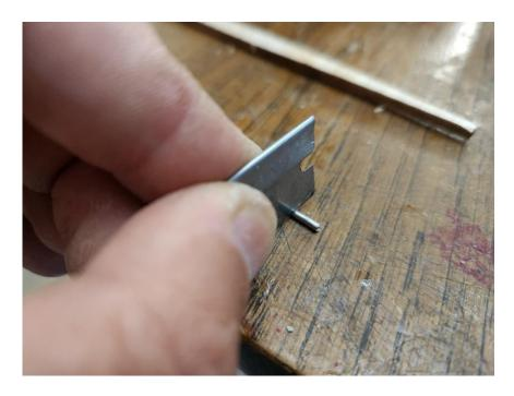
Once the tubing is scored, deeply, it can be broken loose.
