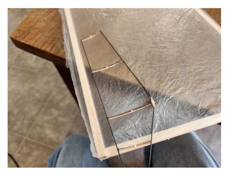
Use an electric cautery (available from indoorffsupply.com) or brand new razor blade to cut the film around the outside of the flying surfaces. Excess covering won't hurt on the leading and trailing edge, as it can be wrapped around the spars, but the tip rib must be trimmed flush.
