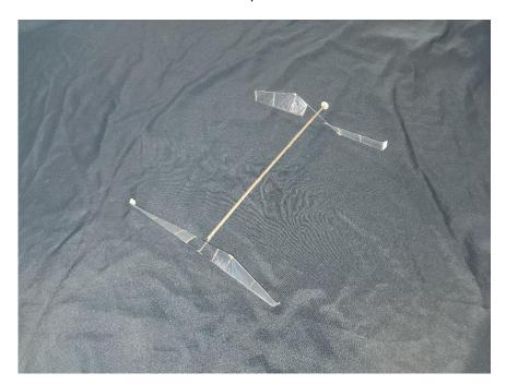
Weigh your model to verify that it meets the minimum weight of 4.00g. If not, glue clay to the top of the motorstick, below the top cap, to bring it up to the minimum weight. The weight will need to be secured with a drop of glue.
