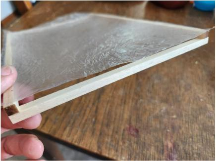
Take your rotor blades outside, or into a spray booth, and spray the convex curved rib side of each with 3M Super 77. This will make them extremely sticky—be careful! It is very easy to damage the parts once they have been sprayed because they will stick to your hands and get damaged if you don't carefully disengage your hands from them.
