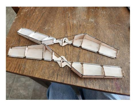
Carefully remove all the tape and gently remove the rotors from the jigs. You may need a razor blade to carefully cut the blades loose in a few places since glue can seep against the jigs.
