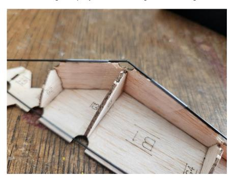
Trim the rod flush with the outside edge as shown.
