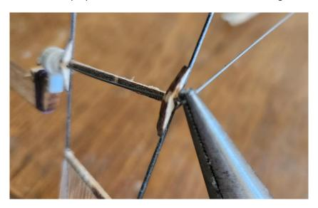
Make another 90 degree bend so that the wire laps over the rotor spar.
