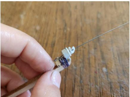
Slide the bottom rotor onto the shaft, curved, covered side toward the motorstick.
