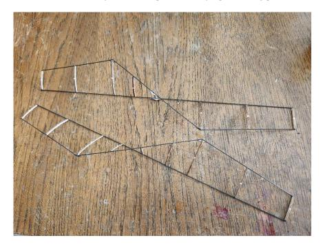
The large  $\frac{1}{2}$ " square sticks are used to make your covering frame. The blade design of this kit requires the covering to be free on the ends of the covering frame. Glue the sticks firmly together to form a rectangular frame by overlapping them as show so that the shorter pieces are offset as shown.
