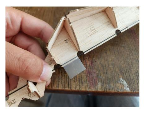
Tape the rod down at the other end of the jig and cut it flush with the outside end of the jig.
