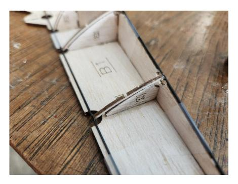
Install the tip rib, to finish out one half of the top rotor.
