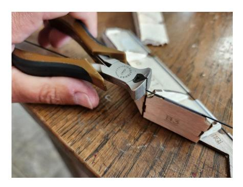
Join up a carbon rod with the segment you just installed, using CA, and holding it down with tape.
