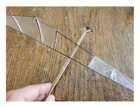
Glue the winglets onto the rotor tips as shown at a roughly 45 degree dihedral angle.
