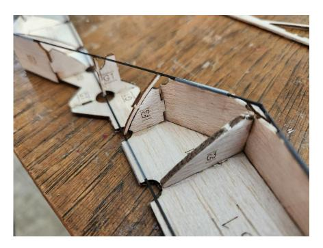
Install the second curved rib (G3 station), resting the front of it on the gusset and securely gluing that junction.
