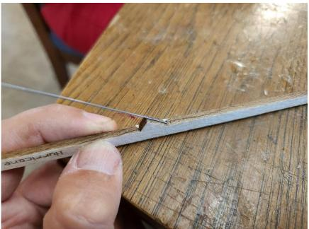
Bind the wire firmly in place and harden with CA.
