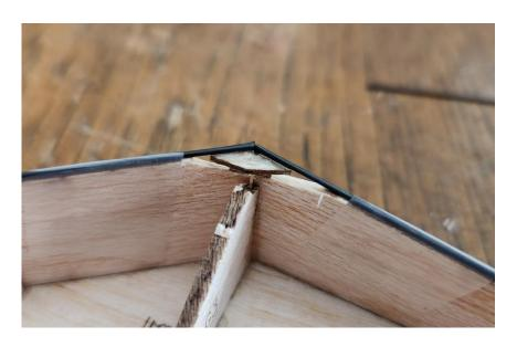
Repeat the above steps for the other side of the rotor so that all of the leading edge is installed on both sides of the jig.
