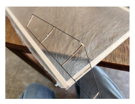
Carefully press the rest of the blade, one rib at a time, down against the film. Take your time to remove wrinkles from the film as you you're your way along. Once the film is fully attached, gently run your finger around the outlines of the rotor to press the film into contact with the parts. Be careful to press very, very gently so that you do not damage the fragile ribs!
