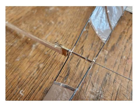
Leaving about 1/8" extra in the prop shaft, bend the wire over SHARPLY to 90 degrees.
