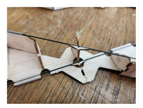
You should now have two completely assembled rotors, taped to their jigs.
