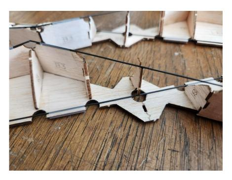
The **bottom rotor requires two shaft alignment plates.** These are the small notched triangles. And they are installed against the spar, lining up the notch with the center rib.
