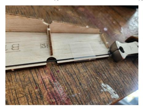
Tape a carbon rod to the top of the jig to form the center leading edge. Make sure the end of the rod is lined up with the centerline of the G3 station.
