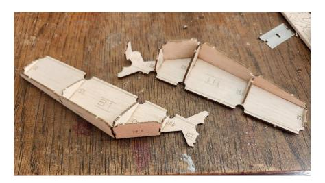
Join the top rotor jig halves together, being sure to keep them flat on the table so that the bottom of the jig remains straight and flat.
