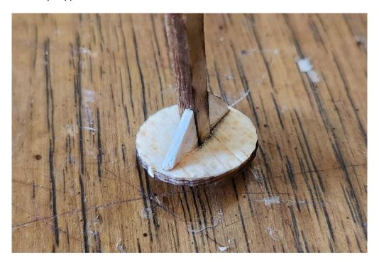
Insert the .020 piano wire into the motorstick, gluing it firmly in place.
