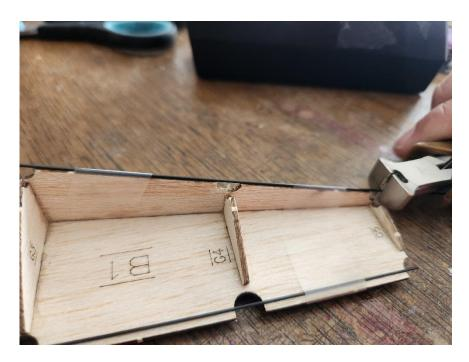
Install one of the rotor leading edge gussets as shown, under the join of the two carbon rods. This is a very small part so you will need to stab it with a razor blade or very thin sewing needle to maneuver it into place.
