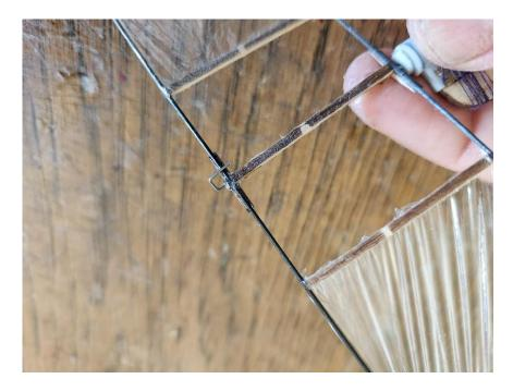
Glue the end of the shaft firmly in place and run glue along the center rib as well. **Don't get glue into the washers or aluminum bearing!!!**
