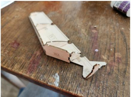
Assemble the second top rotor jig half so that it matches the first one except for the G1 station.
