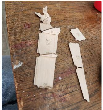
Install the leading edge jigs as shown, again making sure the tabs are fully inserted.
