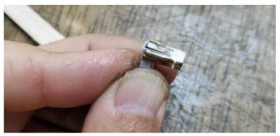
Glue the nose ring assembly in place on the motorstick as shown.
