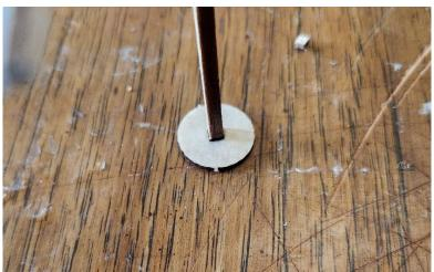
Add gussets on the sides of the cap as shown to prevent it from breaking along the grain (note the grain direction on the top cap).
