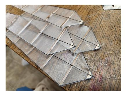
The rotor blades attach to the angled face of the pitch plate and along the wooden spar stub. Make sure they are both firmly attached and exactly aligned with the pitch plate. If your pitch plates are attached in the correct orientation, the order of assembly on blade attachment shown below is noncritical.
