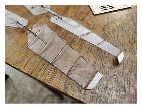
Remove a motorstick from its carrier sheet. Attach the plywood rubber hook as shown. The hook points toward the narrow end of the motorstick.
