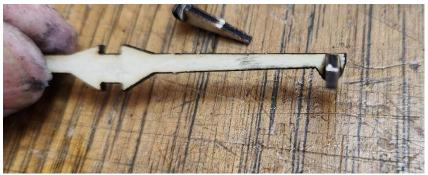
Check the photo below to verify for yourself the correct orientation of the pitch plates. These are necessary to achieve the contra rotating configuration of the rotors.
