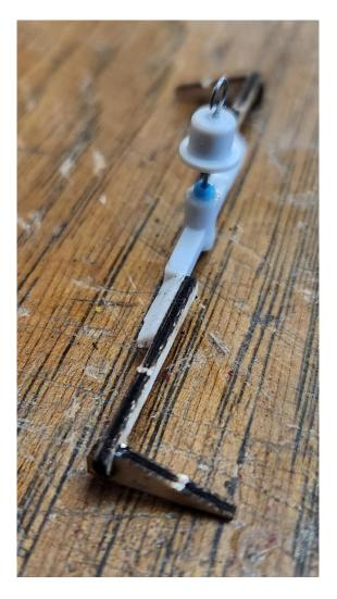
Find the top rotor hub/stub and the corresponding pitch plates. Install the pitch plates in the orientation show.
