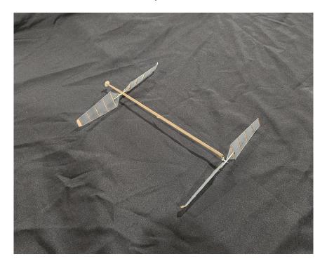
Weigh your model to verify that it meets the minimum weight of 4.00g. If not, glue clay to the top of the motorstick, above the top rotor.
