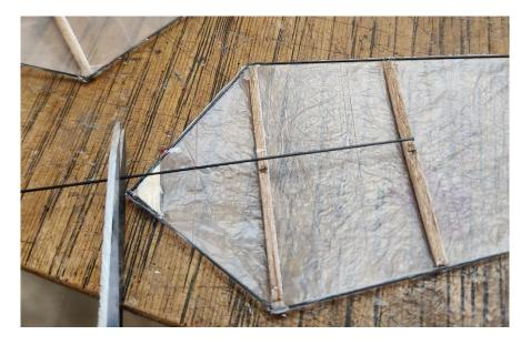
Attach a piece of .020" carbon rod to the bottom of a rotor blade as shown. There are alignment slots in the ribs to show the correct alignment and allow the rod to recess into the rib.
