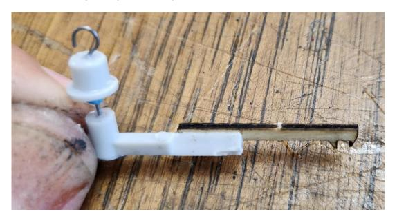
Attach the second bottom spar stub.
