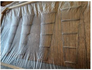
Use an electric cautery (available from indoorffsupply.com) or brand new razor blade to cut the film around the outside of the flying surfaces. Do not leave any excess. Try to get as smooth of a trimming job as possible. Excess film waving in the air will make your model fly poorly.
