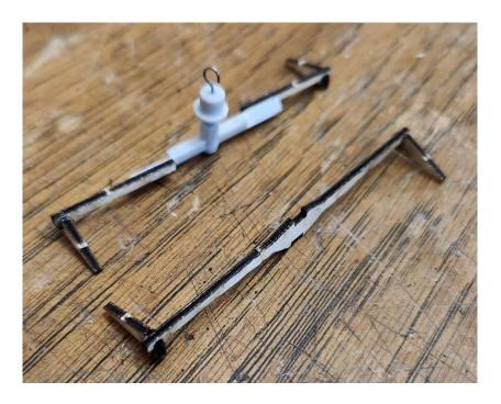
Cut a piece of .020" carbon rod to match the distance between the blade root and the second rib. You will need 4 such segments of carbon rod.
