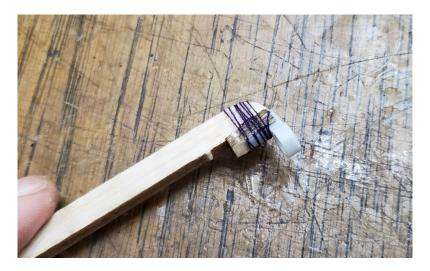
Insert the small end of the motorstick into one of the top caps.
