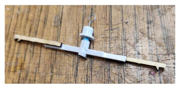
Insert and glue the pitch plates in the ends of the spar stubs facing forward from the hub as shown. This alignment is critical to achieve proper rotation of the rotor so do not get it backwards!
