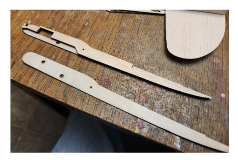
The fuselage side with the large rectangular hole (battery port) is the right side (this allows for correct orientation of the dethermalizer antenna). Glue the fuselage core to this fuselage side.
