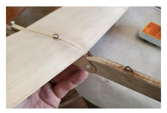
Add the DT hooks in the wing center break and fuselage as shown. Secure these hooks firmly in place with CA glue or epoxy.
