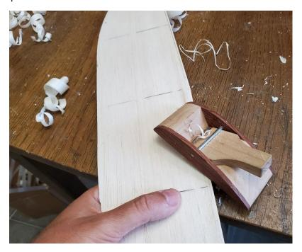
Use your razor plane to taper the lower surface of the leading edge upward to finish the airfoil. The curvature should extend about  $\chi''$  back from the wing leading edge on the lower surface for maximum performance.
