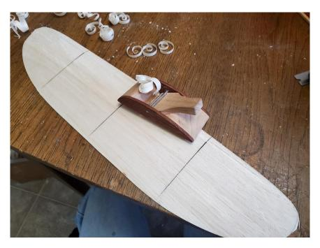
Begin tapering the leading edge with your razor plane. You want a thin rounded section that is almost sharp at the front.
