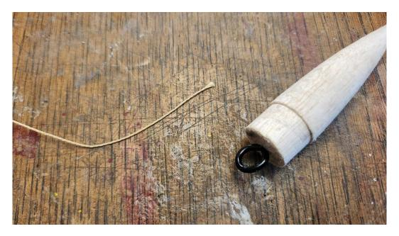
Install the screw eye in the nose cone. Remove the screw eye, squirt glue in the hole, and reinstall.
