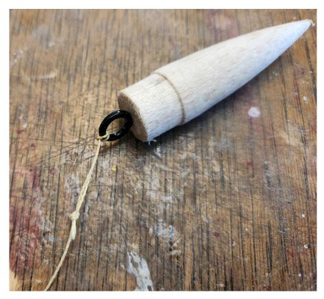
Tie loose the end of the shock cord around the screw eye. Glue the knot so that it cannot come untied.
