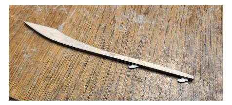
The pod connector saddle is formed by laminating the 1/16" plywood piece with the lug inserts to the 1/8" balsa segment which matches it. Be very careful to get these two components accurately lined up
