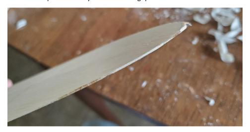
The trailing edge should be about 1/32" thick from the wingtips all the way around to the wing root. Don't sand it thinner than this or it will warp and be easily broken. There is almost zero aerodynamic or weight advantage to going thinner!
