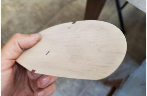
Plane and sand the elevator to an airfoil shape. No upsweep is required in the bottom of the stab leading edge. Don't sand the trailing edge too thin or it will be fragile and prone to warps. The leading edge should be rounded, not sharp, so that it is not easily damaged.
