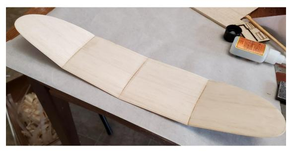
As before, use medium CA or epoxy to join the tips at the correct angle using the dihedral gage. Sand all of the dihedral breaks smooth, and sand a small flat area on the bottom of the wing center dihedral break.
