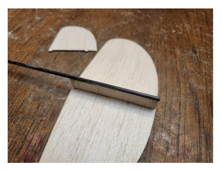
Glue the tailboom to the stabilizer pylon. If a tapered boom is supplied, the tail will attach to the smaller end of the boom. Take your time to get the pylon attached as straight as possible or you will be stuck with whatever turn orientation it ends up with. It's always easier to set the glider for you own desired turn direction later.
