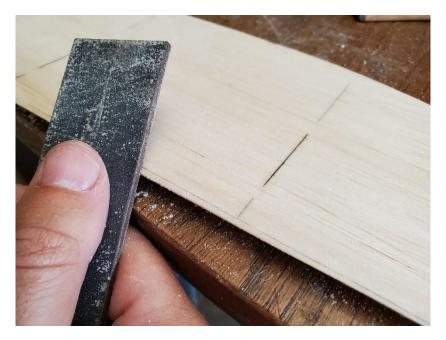
Sand the bottom of the leading edge round as well, fairing in the upsweep you created with the razor plane so that the bottom of the wing is smooth and streamlined and the leading edge is round and devoid of sharp edges.
