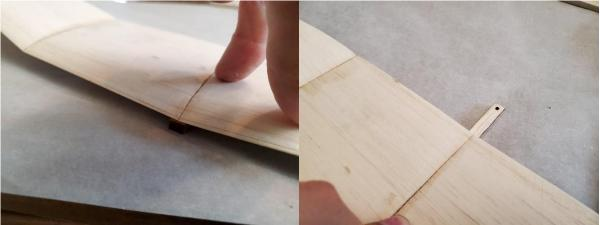
Block up the wing so that it sits level on the wing saddle while you attach the wing to the saddle. The leading edge of the wing is flush with the front of the saddle. The screw hole goes at the back, extending behind the wing trailing edge as shown.
