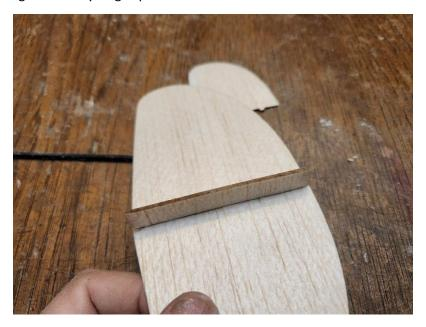
Glue the pylon into the notches on the bottom of the horizontal stabilizer, being careful to keep it straight.
