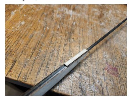
Install the 1/32" plywood wing incidence plate in the back of the fuselage pod over the tailboom.
