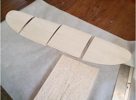
Carefully cut the wing apart at all three dihedral breaks using a Zona saw or similar tool, being careful to avoid tearing the trailing edges. Make clean, straight cuts perpendicular to the wingspan. Note that the tip breaks are skewed. Just follow the cut marks and you will matched skew on each wing, making your glider stall resistant in the glide.
