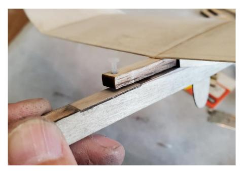
Install the shortened nylon screw in the wing saddle as shown.
