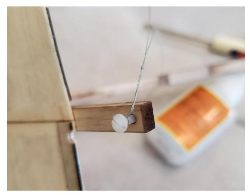
Slip knot this loop around the incidence screw as shown.
