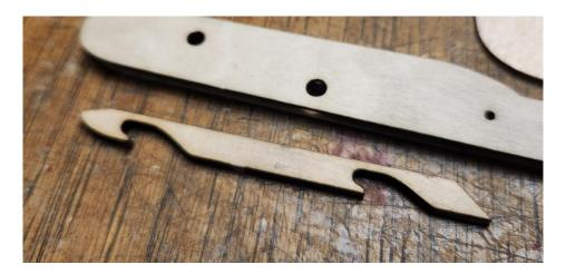
The two narrow fuselage lug pieces (1/16" plywood) must be laminated together. Make sure they are aligned EXACTLY with each other.
