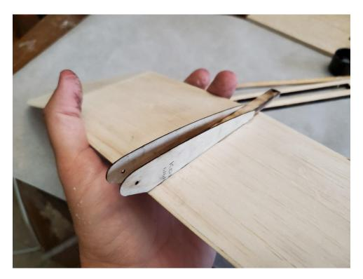
Glue to the wing pivot arms to either side of the wing saddle, with the screw holes facing ahead of the wing leading edge. Be sure to add glue fillets where these arms meet the wing. This bond sees significant loads during launch, DT, and landing.
