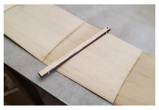
Break the 3/16" balsa wing saddle free from its carrier sheet and sand the laser tabs and burrs off the edges.
