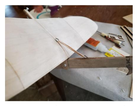
Add a rubber band between the hooks to verify proper DT pivot operation. We have found that the rubber band usually has to be looped around 3 time to get reliable operation.
