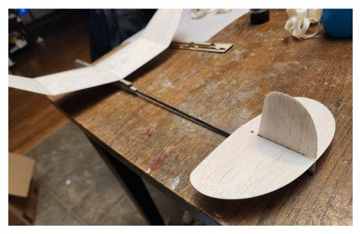
Install the vertical tail in the slots in the horizontal stabilizer.
