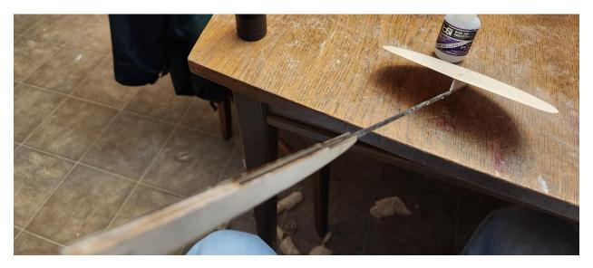
Install the tailboom/tail assembly carefully into the fuselage. Get the stabilizer as close as possible to perpendicular to the fuselage side profile.
