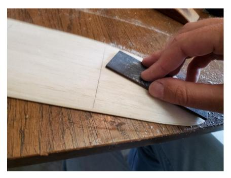
Sand the entire upper surface of the wing as smooth as possible using 300-600 grit sandpaper. Leave the trailing edge thickness alone with no rounding, but sand the leading edge smooth and streamlined. Sand until all gouges are removed.
