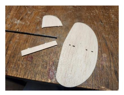
Sand the stabilizer pylon and fin to streamlined cross sections. Be very careful to avoid breaking the pylon during sanding as it is very fragile prior to installation.
