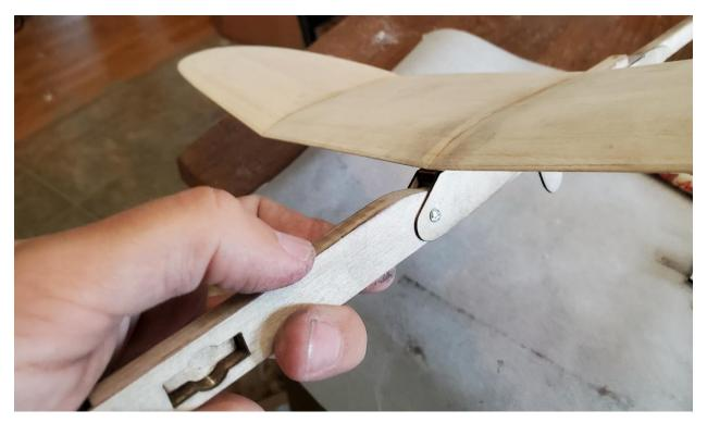
Install the wing on top of the fuselage using the 2-56 steel screw. Sand the fuselage in front of the wing as needed to get at least 60 degrees of forward travel in the wing, and sand the fuselage area that is covered by the pivot arms until there is minimal resistance to the wing pivoting from its flight position.
