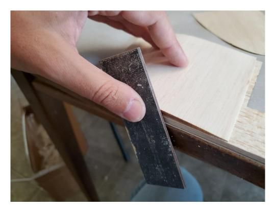
The dihedral breaks are around about 16 degrees at the tips and 10 degrees in the center, so use the edge of a table and a good straight sanding block to sand the dihedral breaks to about 8 degrees on each surface and 5 degrees each surface at the center.
