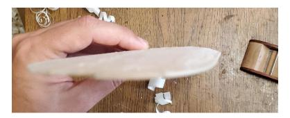
Only plane down until the balsa is flush with the basswood liner. You will taper the bottom of the leading edge up to provide the rest of the airfoil.
