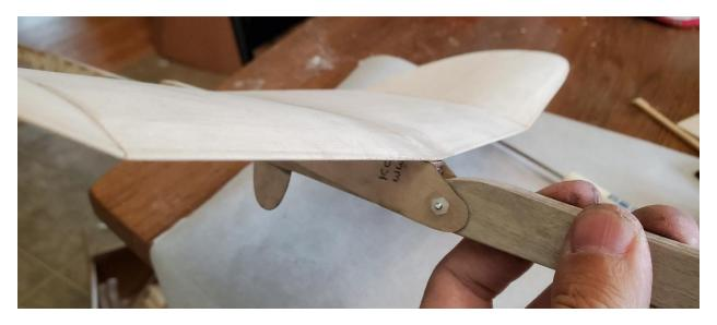
The steel screw is held in place with a nylon nut.
