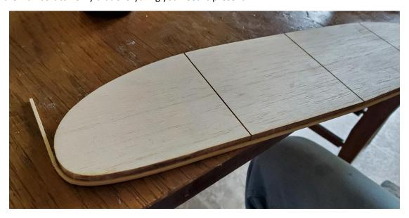
Break the wing out of its carrier sheet (don't throw away the remaining laser cut part in this sheet) and sand the edges smooth of any tabs and burs. Wet out the 1/16" sq basswood strip and glue them to the
