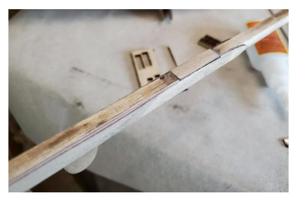
Sand the area where the wing will rest smooth and round the top edges of the fuselage thoroughly in this area.
