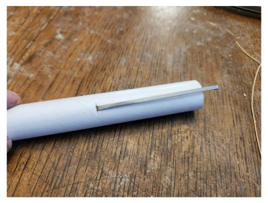
An engine clip suitable for Estes, Quest and Aerotech 18mm motors is included in your kit. If you choose to use it, slot the body tube so that the clip extends about ¼" from the end of the body tube.
