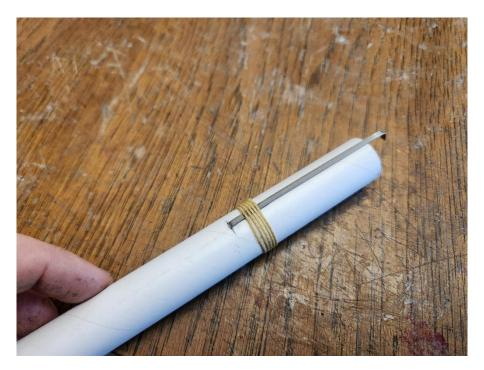
Bind the end of the engine clip with Kevlar and seal with CA glue to retain it. Don't use too much Kevlar, as you will use the remaining Kevlar as a shock cord.
