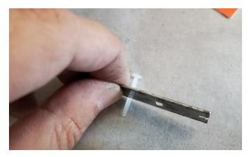
Cut the nylon 2-56 screw to 2/3 of its supplied length using a razor blade.
