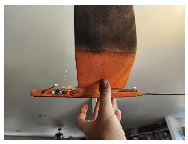
Install the dethermalizer timer using a small servo screw, being careful to avoid damaging the battery connector, which can be quite vulnerable. If necessary, widen the hole for the battery so that its leads can be threaded through. It will be necessary to tape the battery in place. You can now balance your Polly Rocket glider. Starting CG is 50% of root chord (half of the way back from the leading edge). Turn the incidence screw in 1 turn from flush with the bottom of the saddle to start.
