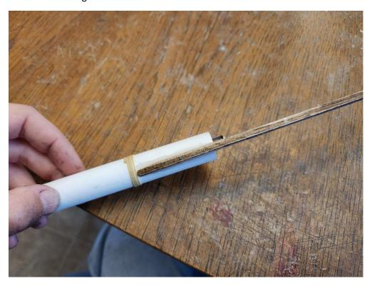
Sand the attachment area of the glider connector and glue it to the body tube.
