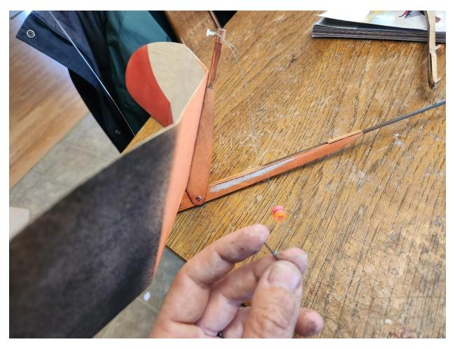
Remove the wing DT rubber band so that the wing can be laid in the glide position without force. Loop the DT line around the fuselage, around the incidence screw, and forward under the wing to the timer. Tie off a piece of carbon rod about 3/8" short of the timer so that a DT band can be stretched over the timer from this carbon crossbar retainer you have created.
