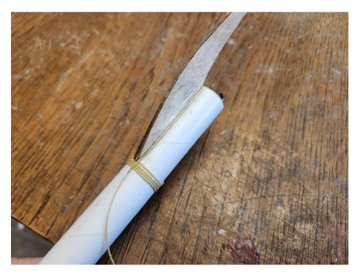
Run the Kevlar shock cord material around the back of the connector and glue it in place in a fillet.
