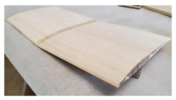
Use a thorough coat of medium CA glue or epoxy to join the center section.
