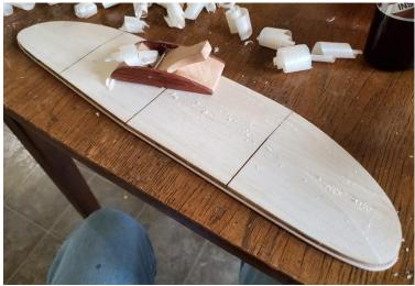
Use your razor plane to carve the trailing edge to a shallow bevel. Take your time to gradually progress the bevel across the trailing edge. Your goal is to create the trailing edge profile shown below:
