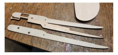
Break the fuselage core out of its carrier sheet with extreme caution as the front is quite fragile. Also break out the 1/32" plywood sides.
