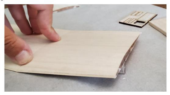
The short dihedral gage is used for the wing center section join.
