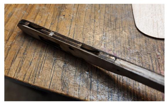
Insert and cement the fuselage lug pieces into the bottom of the fuselage. Be careful to ensure proper orientation.
